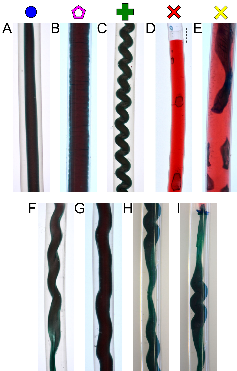
Fig. 1 Examples of precipitation patterns obtained in the co-flow system: A straight tube, B worm-tube, C helix, D unsuccessful experiment where the bubble (visible in the upper part inside the dashed rectangle) has taken a cylindrical shape, and E failed experiment where the bubble was trapped between the inner and outer FEP tubes. The precipitation occurred without the presence of a bubble. F–I Various forms of helices obtained. The scales of the photos are given by the outer diameter of the outer tube d_{\text{out}}^{\text{Si}} = 3.2 \text{ mm}
