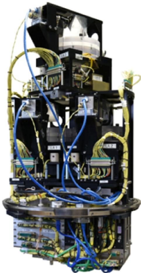
**Fig. 8 | Photograph of the CDIC-4 module.** The experimental units are visible, one on top and two at the bottom. The electronics compartment is also visible at the very bottom part of the image. The image is a courtesy of AIRBUS Defense and Space.
