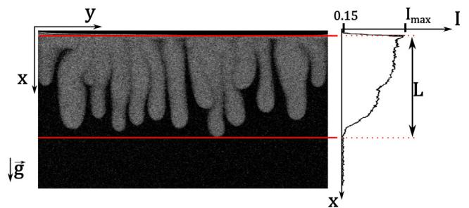
**Fig. 4.** Processed image of  $\text{CO}_2$  fingers in BP solution at  $t = 30$  min and corresponding TAP along the  $x$  axis. The finger length  $L$  is computed as the length of the region where TAP decreases from its maximum value  $I_{\max}$  (the interface) to 0.15.
