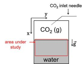
**Fig. 1.** Schematic representation of the system. The cell is partially filled with deionized water and gaseous CO<sub>2</sub> is introduced through the top of the cell using a narrow needle inserted between the glass plates.
