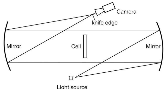
**Fig. 8.** Schematic of the Z-type Schlieren system used to visualize buoyancy-driven convection of CO<sub>2</sub> in NaOH solutions. Our set-up is composed of two 20 cm diameter mirrors with 1 m focal lengths. The Hele-Shaw cell is placed between the two mirrors and a CCD monochromatic camera records the dynamics at successive times.
