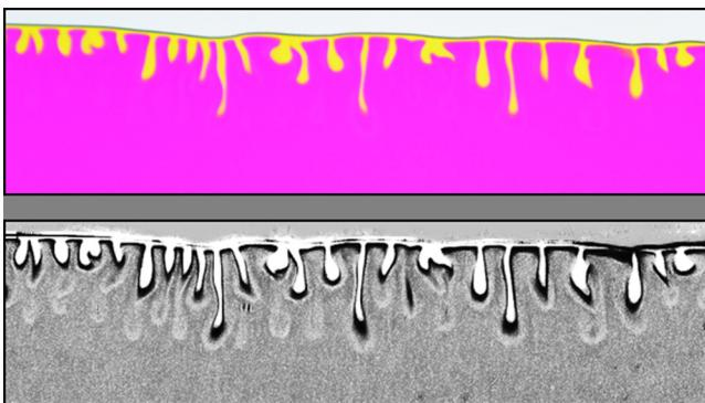
**Fig. 10.** Comparison of  $\text{CO}_2$  convective dynamics at  $t = 300$  s in a solution of  $\text{NaOH}$  ( $1.000 \times 10^{-2}$  mol/L) containing phenol red ( $5.0 \times 10^{-4}$  mol/L) by direct visualization of color changes (up) and by Schlieren visualization (down). (For interpretation of the references to color in this figure legend, the reader is referred to the web version of this article.)
