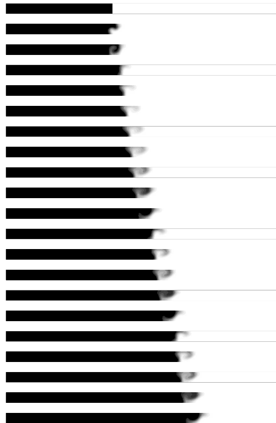
FIG. 5. Oscillatory propagation of the concentration front in the presence of competing solutal and thermal buoyancy effects for R_C=-10 , R_T=15 , and Le=5 shown from top to bottom from t=0 up to t=60 with a time interval of \Delta t=3 ( V=1.50 ). The initial condition is at x=100 and the aspect ratio between L_x=256 and L_z=10 is preserved.
