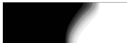
FIG. 6. Concentration field in the moving frame obtained by numerical integration of the simplified equation [Eq. (27)] for L_z = 10 . The aspect ratio between L_x = 30 and L_z is preserved.
