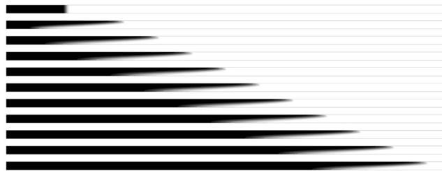
FIG. 2. Propagation of a chemical front in the presence of chemically induced buoyancy convection for Ra=100 , shown from top to bottom from t=0 up to t=50 with a time interval of \Delta t=5 . The aspect ratio between L_x=450 and L_z=10 is preserved.
