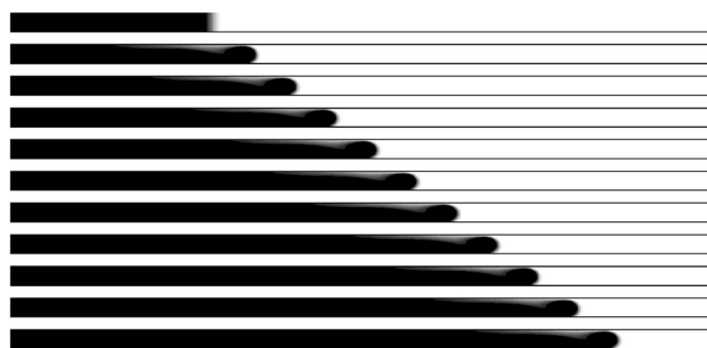
FIG. 13. Propagation of a chemical front in the presence of chemically induced Marangoni convection with apparition of an additional deformation for M=-1000 . The dynamics is shown from top to bottom from t=0 up to t=50 with a time interval of \Delta t=5 . The aspect ratio between L_x=350 and L_z=10 is preserved.
