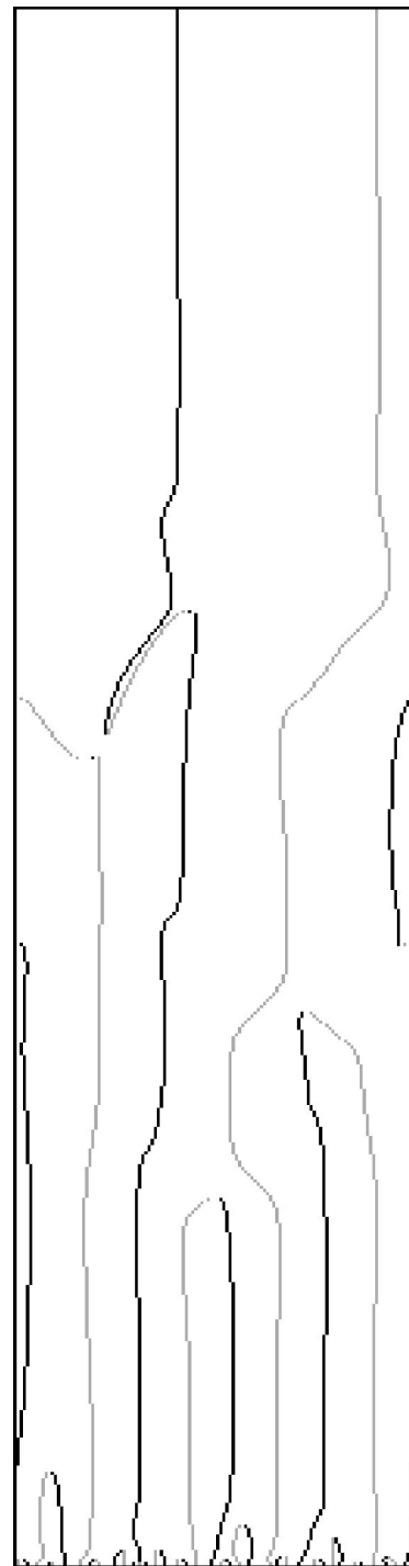
FIG. 10. Space-time map of the locations of the maxima (black) and minima (gray) of the transverse averaged profile \langle c(y,t) \rangle as a function of time for simulation of Fig. 3(a) ( Ra=512 , Da=0.01 , d=0.01 ). The horizontal direction corresponds to the y coordinate while the vertical axis is time running upwards.
