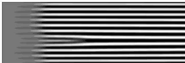
Figure 1. Space–time diagram showing the development of a periodic spatial pattern. Time runs along the horizontal axis, and the spatial coordinate is plotted along the vertical axis. The size of the one-dimensional system is L = 20 , and the displayed time interval is T = 50 . Local concentration of species C is displayed in gray scale, with brighter areas corresponding to higher concentrations. The model parameters are P_A = P_B = D_A = D_B = D_C = 1 , c = 0.5 , \epsilon = 5 , r_0 = 0.2 , and w = 0 .
