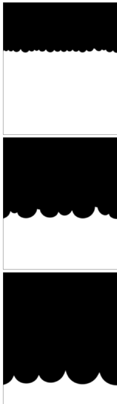
FIG. 6. Density plot of the fingering instability at various times for Da = 0.005 , \kappa = 1 , Ra = 1024 , and \delta = 1 . The initial condition is a step function. The system is shown from top to bottom at three successive times t = 600 , 900, and 1200.
