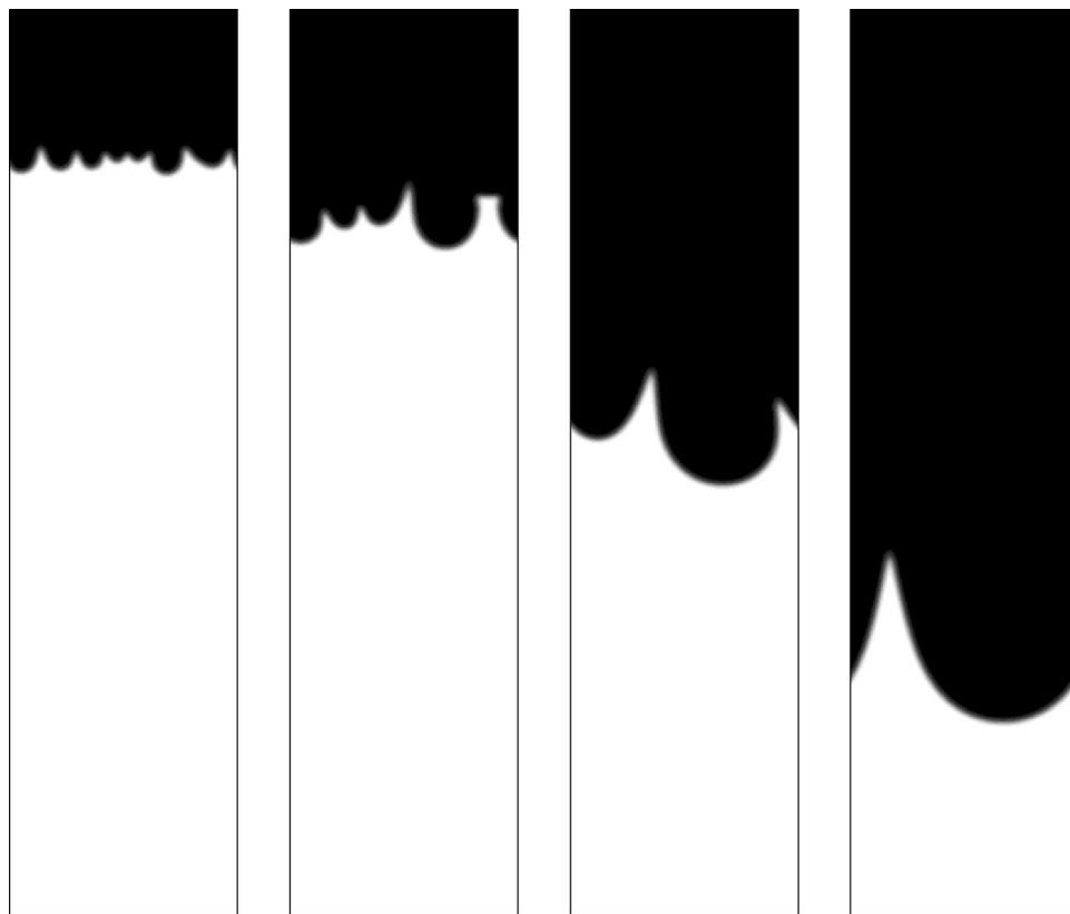
FIG. 7. Density plot of the fingering instability at various times for Da = 0.001 , \kappa = 1 , Ra = 512 , and \delta = 1 . The initial condition is a step function. The system is shown from left to right at four successive times t = 900 , 1200, 2100, and 3000.
